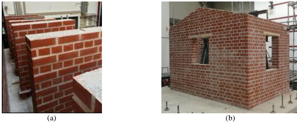
Figure 1. Experimental campaign: (a) walletts for compression tests, and (b) real scale construction for shaking table tests.
