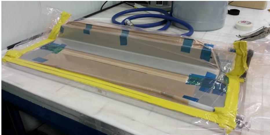
Figure 4: VARTM setup with rigid tooling
