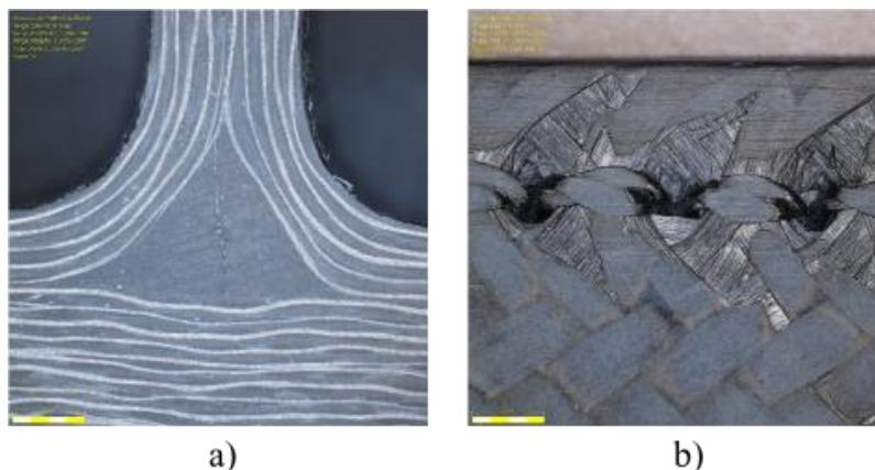
Figure 8 Optical inspection: a) Noodle area b) Resin poor zones near stitching
