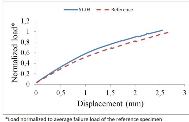
Figure 10: Average load-displacement curves for asymmetric tear-off test
