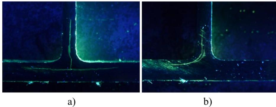
Figure 9 General crack propagation path: a) Symmetric loading b) Asymmetric loading
