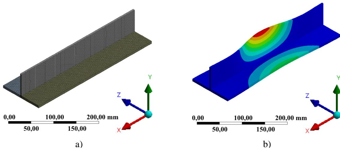
Figure 7 Finite element model of column: a) Meshing b) predicted buckling mode
