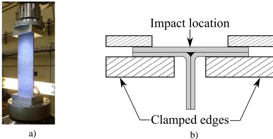
Figure 6 Test setups: a) Compression setup b) Impact rig setup
