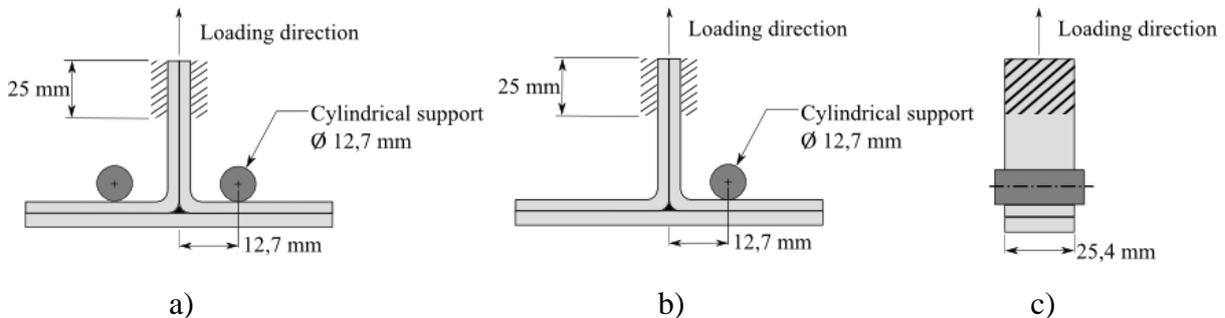
Figure 5 Tear off test: a) Symmetric test b) Asymmetric test c) Side view
