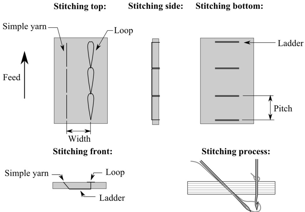
Figure 2: Illustration and nomenclature used for One-Sided-Stitching®
