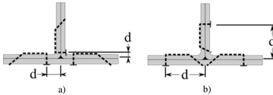
Figure 3 Stitching orientation: a) Adjacent stitching b) Opposite stitching
