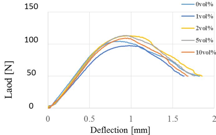
Figure 1 Load-deflection curve for nanoparticle filled and unfilled CFRP specimen.
