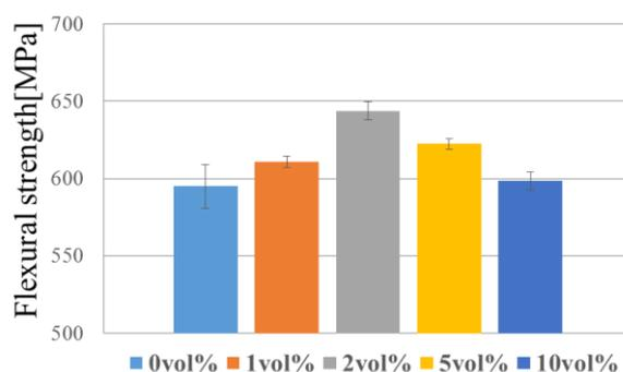
Figure 2 Flexural strength for nanoparticle filled and unfilled CFRP specimen.
