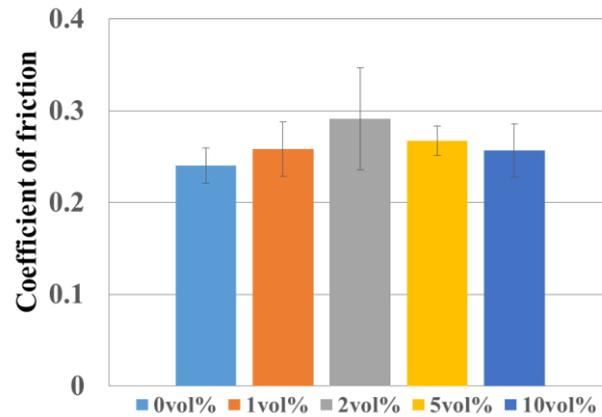
Figure 4 Coefficient of friction for nanoparticle filled and unfilled CFRP specimen.
