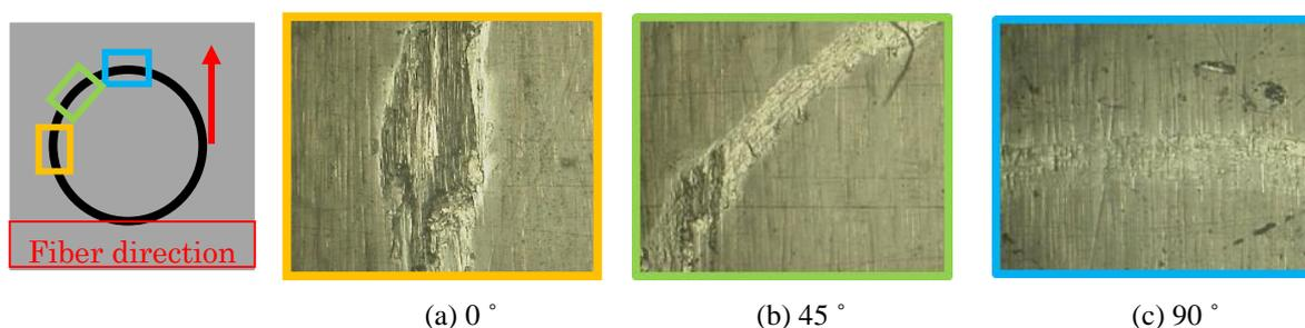
Figure 3 Typical wear test results for the nanoparticle unfilled CFRP specimen (0 vol%).
