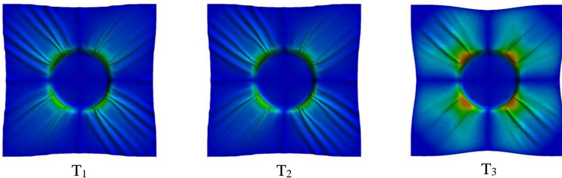
Figure 1: Simulation of a cylindrical forming at different temperatures ( $T_1 < T_2 < T_3$ ).
