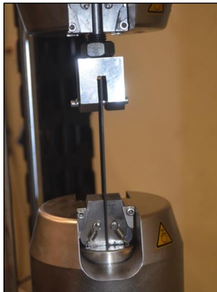
Figure 8 – Specimen in the fatigue testing machine.
