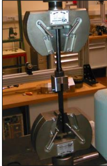
Figure 4 - Specimen fixed in the lower end with pin in double shear insert.
