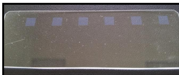
Figure 2: TiO 2 /indicator thin films prepared by depositing the 18NR-T Transparent Titania Paste from Dyesol onto a glass substrate through the screen printing method
