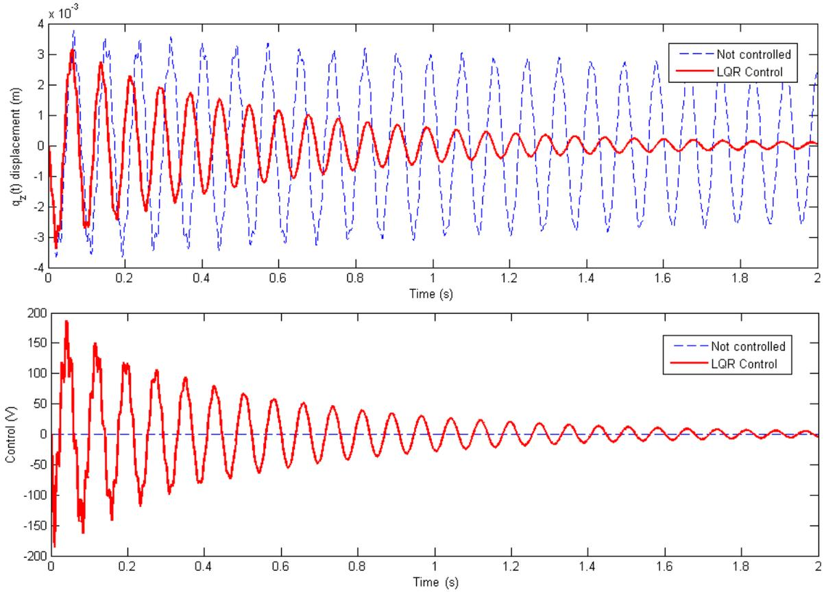
Figure 2: Time response for tip displacement and control force.
