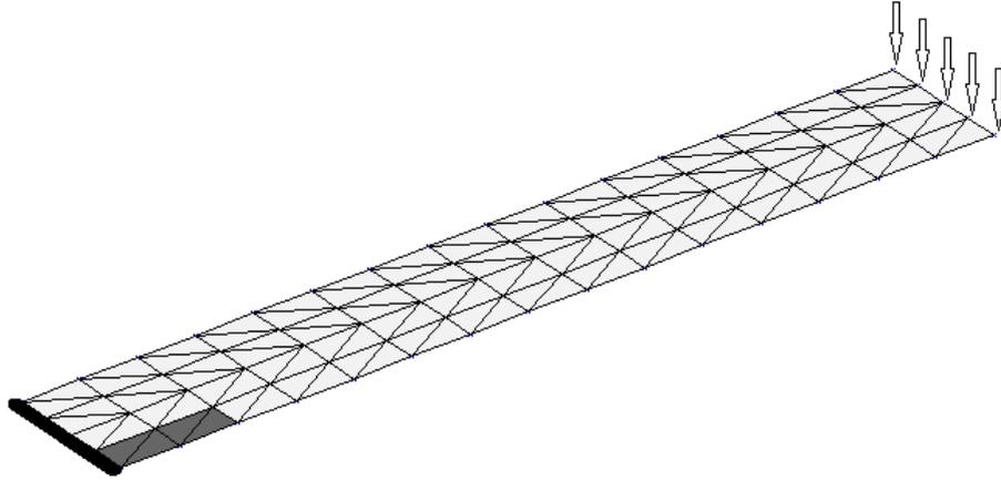
Figure 1: Finite element mesh of the cantilever composite plate with location of the collocated piezoelectric actuators (dark elements) and the location of applied forces.
