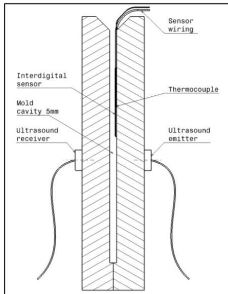
*Figure 2: Cross section of the tooling and sensor positions*
