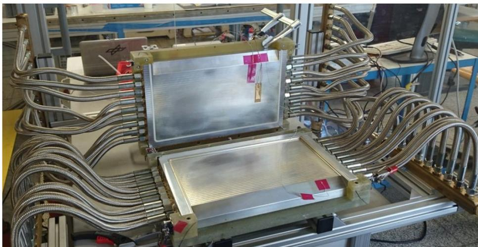
*Figure 3: Opened temperature controlled tooling with sensors attached to the tooling face*
