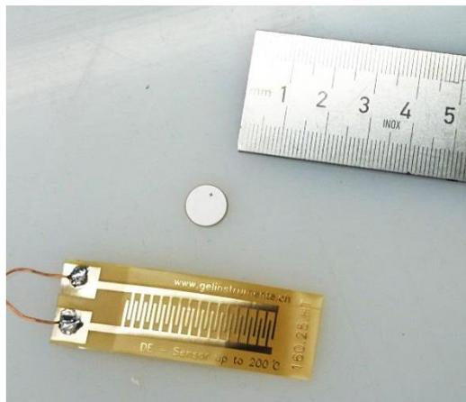
Figure 1: Flat interdigital sensor and above discoidal piezoelectric sensor
