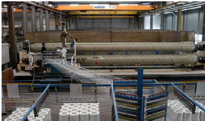
Figure 1: Helical filament winding used in Composite Pipes Industries (CPI) Oman
