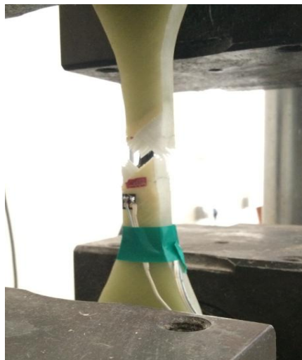
Figure 12: Failed tensile test specimen
