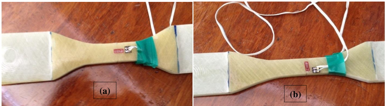
Figure 10: Benchmark pipe specimens prepared for tensile testing of with (a) Axial, (b) Transverse strain gages
