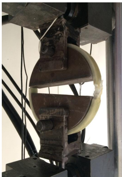
Figure 13: Failed split-disk specimen
