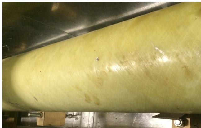
Figure 2: A GRE pipe used in this study with a winding angle of \pm 55^\circ .
