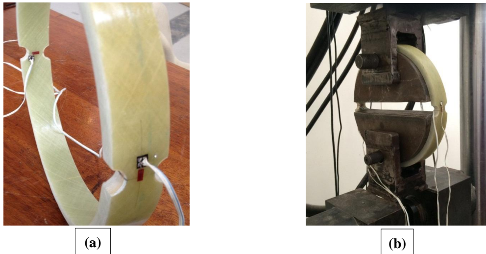
Figure 11: Specimen for Split-disk test (a) with strain gages attached axially and circumferentially, (b) Split-disk specimen with fixtures
