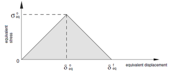
Figure 10: Equivalent stress vs. equivalent displacement [4].
