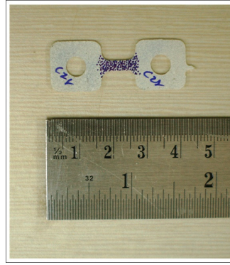
Figure 4: Speckle pattern on glass/epoxy specimen.
