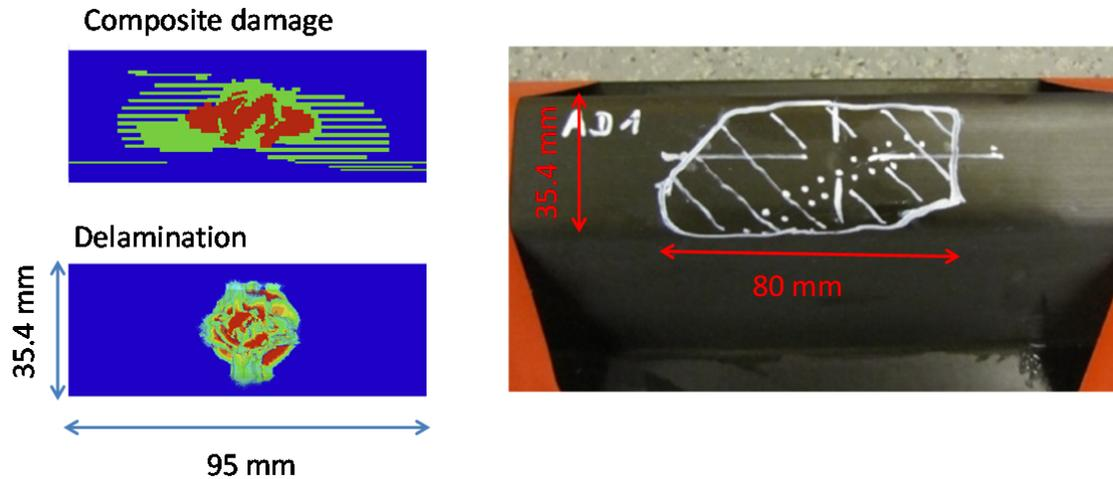
Figure 7 Damage prediction of impacted composite stiffener
