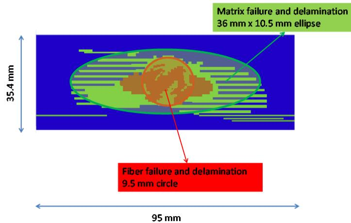
Figure 9 Impact damage idealization
