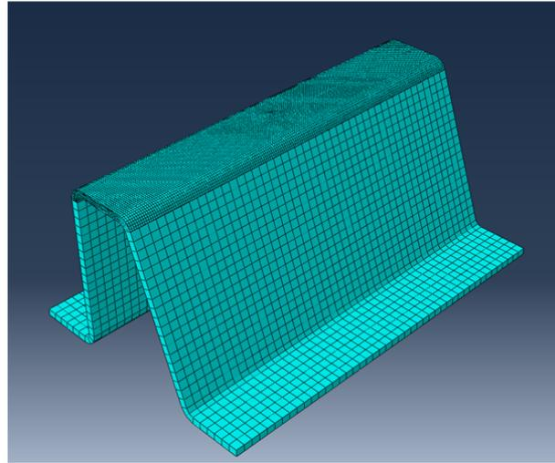
Figure 5 Finite element model of composite stiffener
