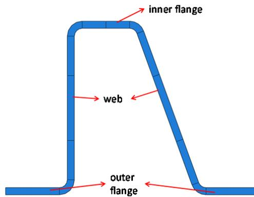
Figure 2 Omega frame cross section
