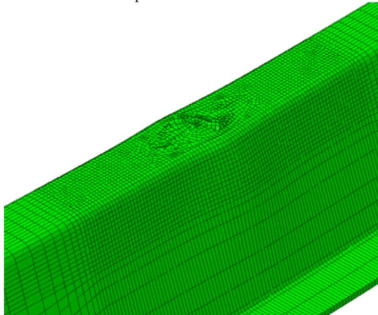
Figure 10 Predicted deformation after 4 point bend test
