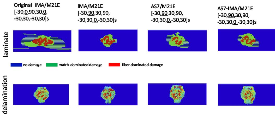
Figure 11 Comparison between impact damage in a composite frame with the original configuration and various other configurations
