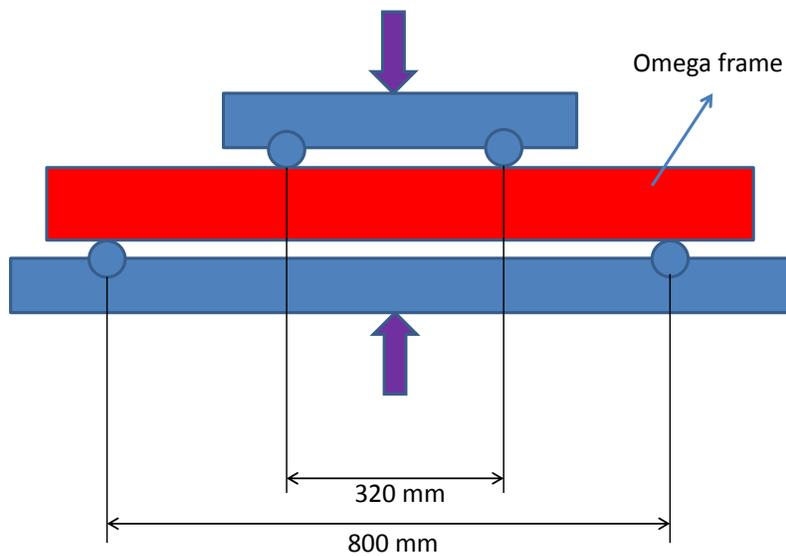
Figure 4 Schematic of four-point bend test
