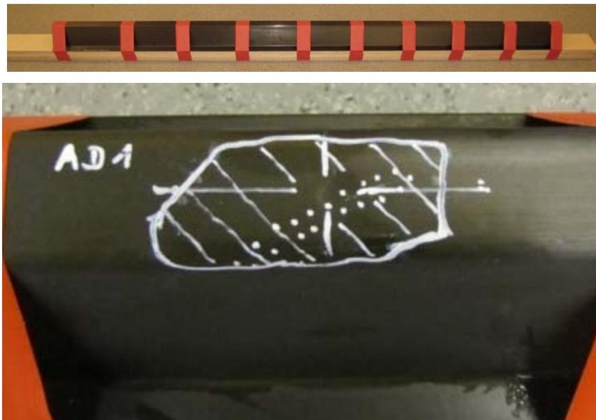
Figure 3 Impacted omega frame
