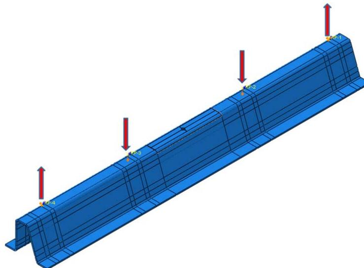
Figure 8 Four-point bend test model
