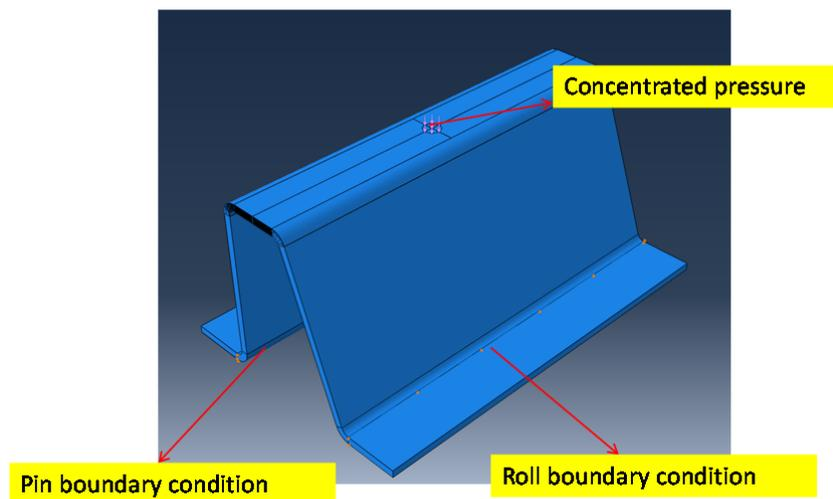
Figure 6 Load and boundary condition
