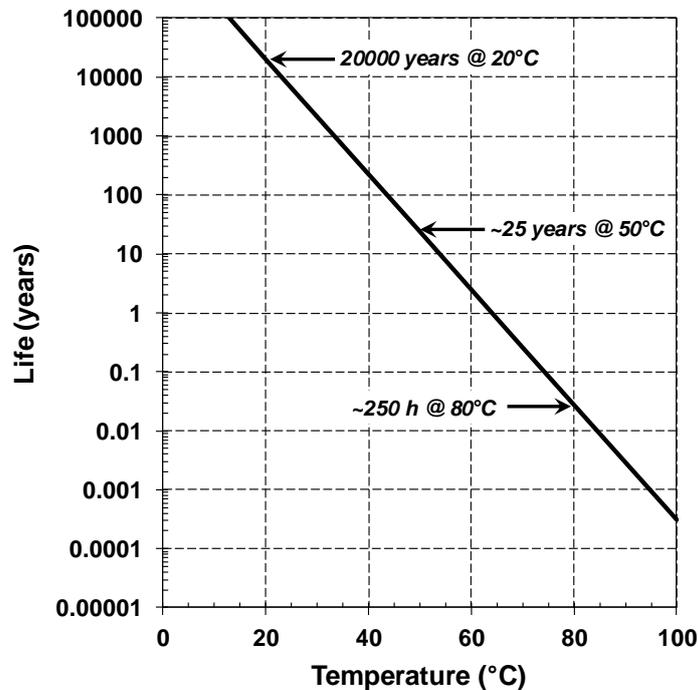
Figure 6: VPPMC life as a function of ambient temperature, based on a time-temperature equivalent of 20000 years at 20°C. Redrawn from Ref. [23].
