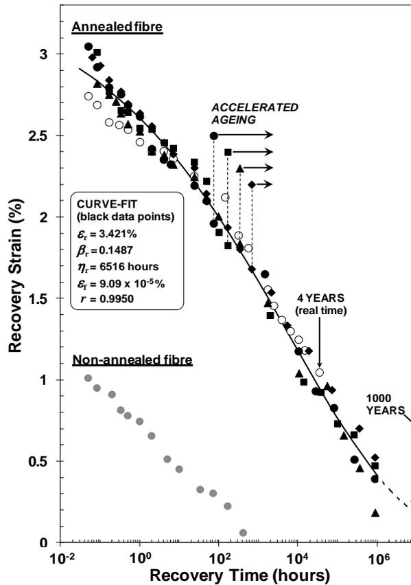
Figure 5: Recovery strain data at  $20^\circ\text{C}$  from nylon 6,6 yarn after being subjected to 24 h creep at 342 MPa. For fibre annealed prior to creep, white data points were measured in real time; black data points are from four samples subjected to periods of accelerated ageing, with curve and parameters from Eq. (1), where  $r$  = correlation coefficient. After Refs. [20, 21].
