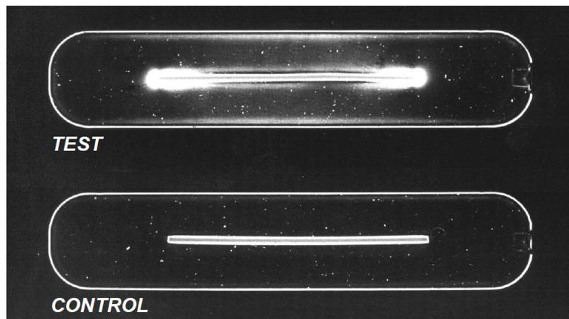
Figure 2: Nylon 6,6 monofilaments (1.6 mm diameter) in polyester resin samples ( $150 \times 30 \times 2$  mm) under cross-polarised light. Note the stress pattern from viscoelastic recovery in the ‘test’ sample, compared with the (unstressed) ‘control’ sample. Image first published in Ref. [17].
