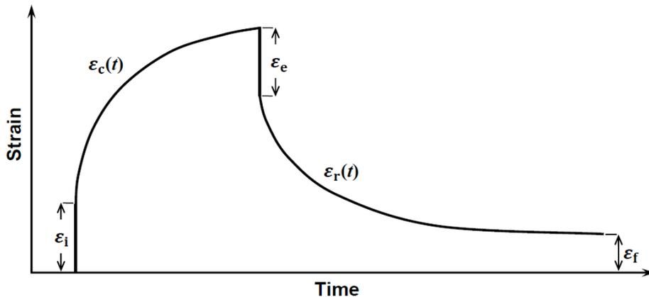
Figure 1: Schematic tensile creep-recovery strain cycle for a polymeric material.
