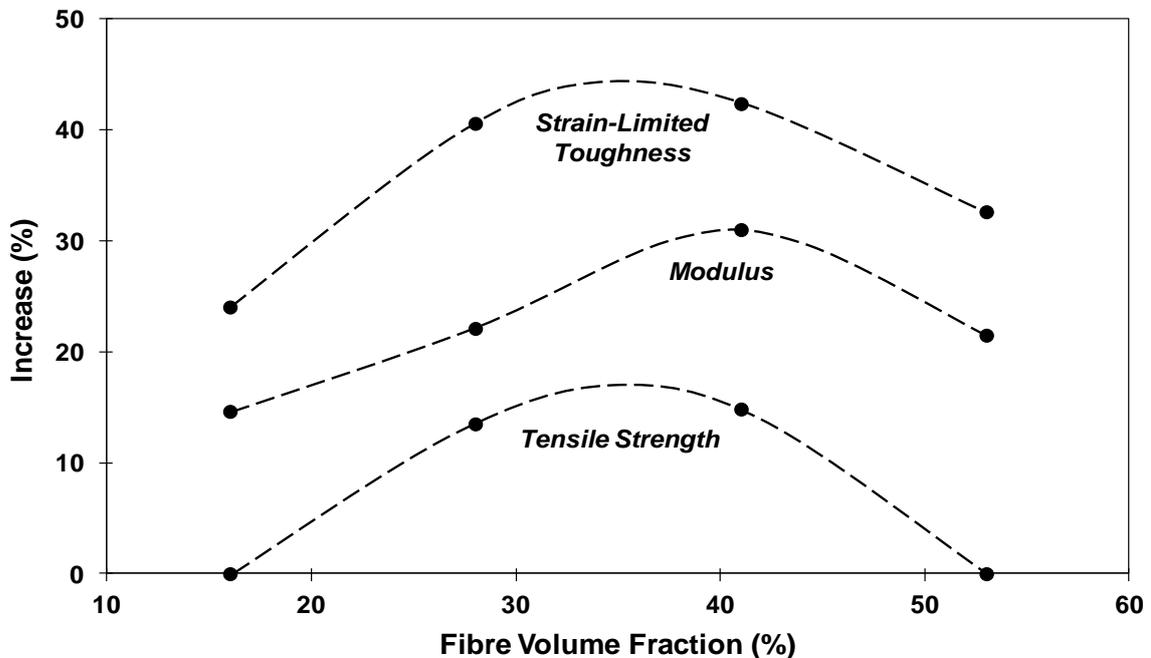
Figure 4: Effect of fibre volume fraction on the measured tensile properties of test (VPPMC) samples relative to their control counterparts. Strain-limited toughness represents energy absorbed/unit volume to a fixed strain (0.25), from area under the stress-strain curve. Redrawn from Ref. [26].
