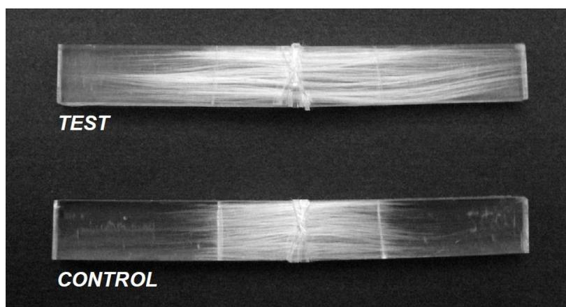
Figure 3: Typical appearance of test (VPPMC) and control (unstressed) samples after impact testing; note the greater region of fibre-matrix debonding in the test sample.
