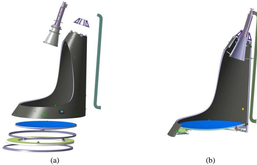
Figure 3: Components of the antenna (a) and a longitudinal section of the antenna (b).
