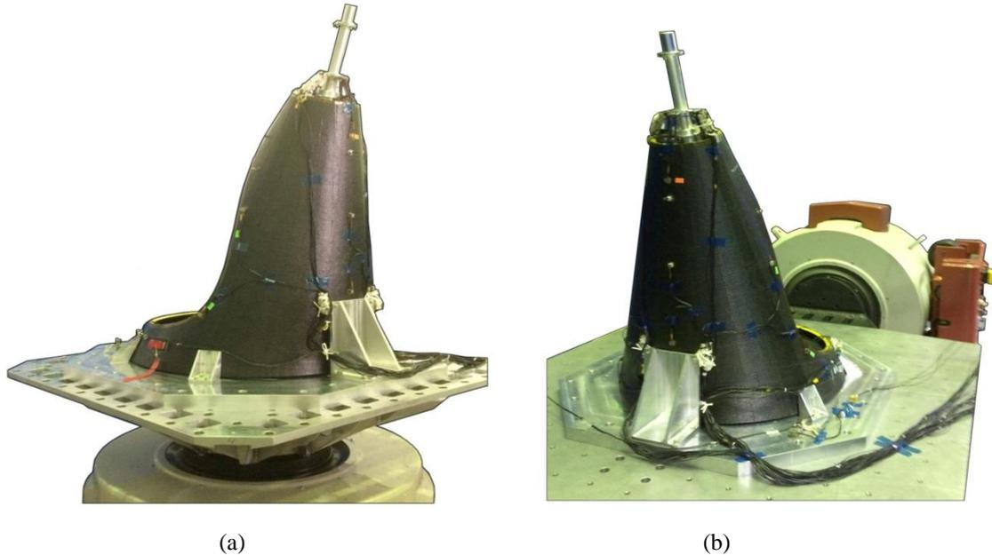
Figure 9: Antenna on the vertical (a) and horizontal (b) vibration tables.
