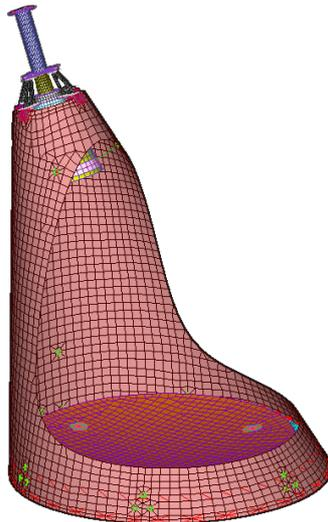
Figure 7: Finite-element model of the antenna.
