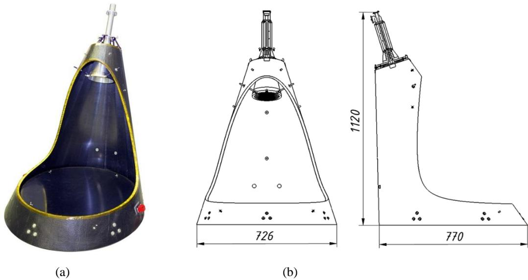
Figure 6: Assembled antenna (a) and dimensions of the assembled antenna (b).
