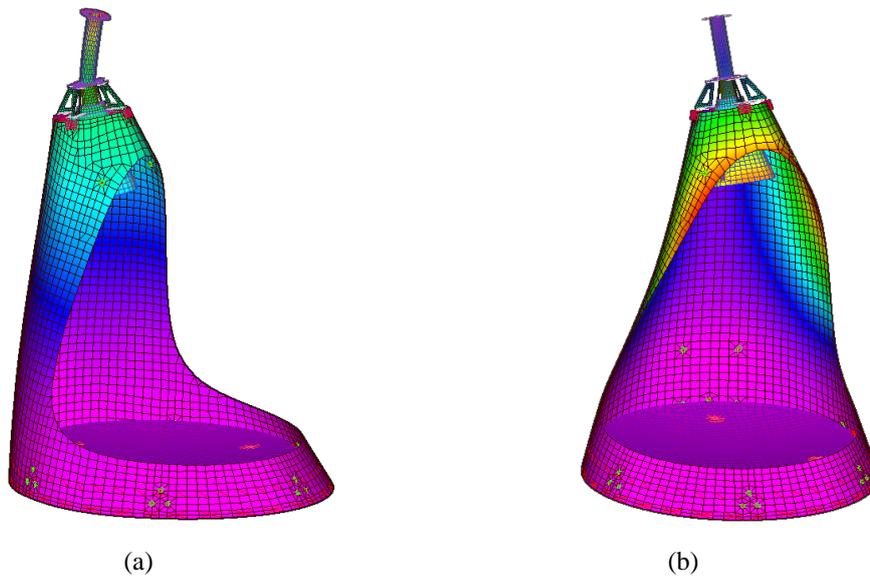
Figure 8: The first (bending) (a), and the second (torsion) (b) vibration modes.
