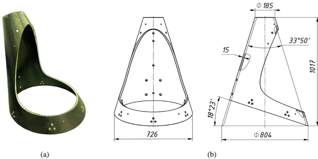
Figure 5: The trimmed sandwich shell (a) and the shell dimensions (b).
