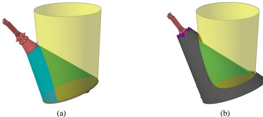
Figure 2: Area of the radio wave transmission (a) and antenna's body covering the transmission area (b).
