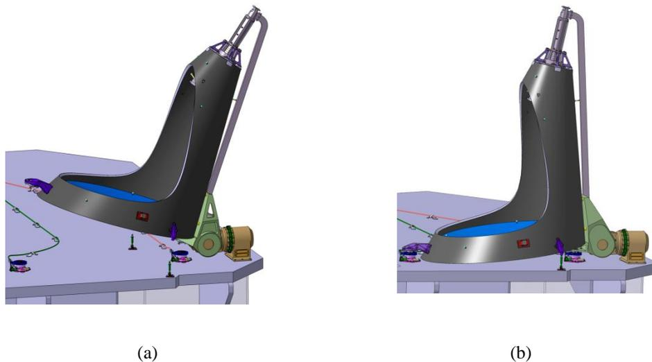
Figure 4: Antenna with the pointing drive (a) and antenna fastened to a spacecraft (b).
