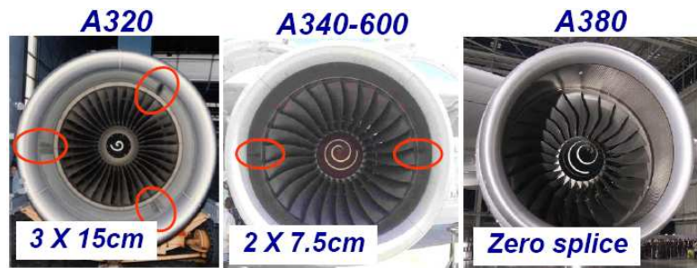
Figure 7: Improved manufacturing techniques fulfills the zero-splice intake liner [5].
