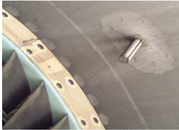
Figure 6: Installation of hard wall forward acoustic-panels (HWFAP) of CFM56 engine.
