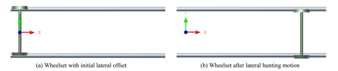
Fig. 3: Autodesk Inventor addin to move wheelset on rails demonstrating kinematic hunting behavior
