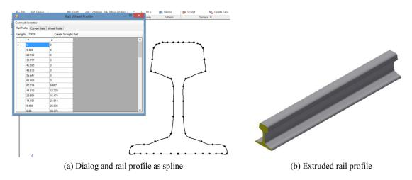
Fig. 1: Inventor addin to create rail using extrusion feature
