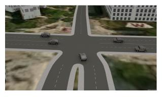
Fig. 2: Chrono:: Vehicle Left: simulation of follow the leader convoy. Right: simulation of DSRC controlled intersection using 30 autonomous vehicles.
