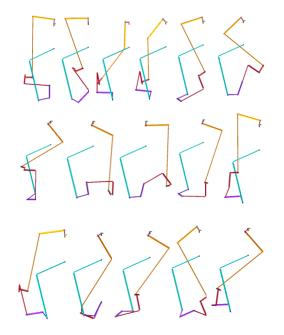
Fig. 2: 3D representation of the 16 distinct inverse kinematic solutions
