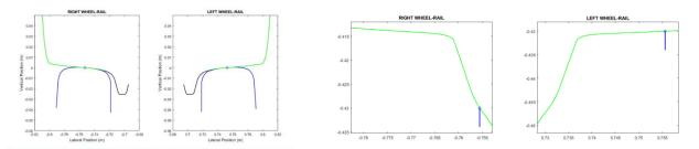
Fig. 1: Wheel-rail profiles in contact (left) and equivalent KEC-profiles
