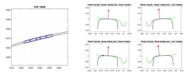
Fig. 3: Simulation of Metro de Sevilla. Top view of the train (left) and computed wheel-rail contact forces (right)
