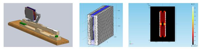
Fig. 2: Design of one-key active feedback device : 3D current CAD view (left) - FEM mesh in  $COMSOL^{(R)}$  of the voice coil actuator (middle) - Magnetic field in the system (right)
