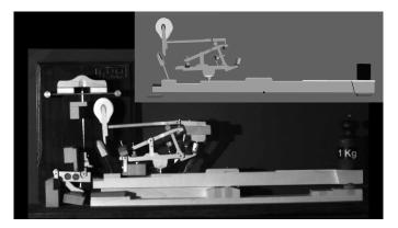
Fig. 1: Motion snapshot of the double escapement piano action and its corresponding multibody model (upper right corner) (from [3])
