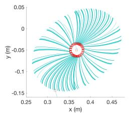
(a) The trajectories of center of mass of the pushed object in experiment data.
