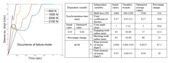
Figure 2: Sleeve axial displacement with varying shift force.
