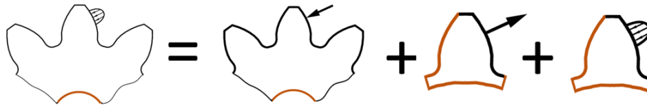
Fig. 4: Computational steps to represent gear total deformation [4].
