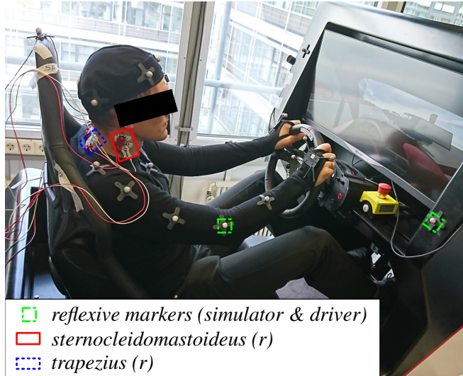
Fig. 6: Sensor placement and marker based skeleton reconstruction. Left: Setup with reflexive markers, i.e. elbow marker (green dash-dotted) and EMG sensors right sternocleidomastoideus (red) and right trapezius (blue dashed). Right: Reconstructed model of the skeleton based on the position data of the markers.
