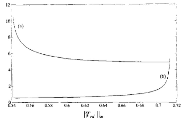
Fig 4.4: The tradeoff between  $L_2$  and  $H_\infty$  performance: (a)  $\|T_{rd}\|_2$ ; (b)  $\gamma$ .
