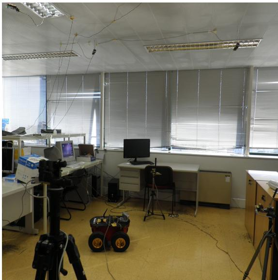
FIGURE 2.9: The test environment and Pioneer P3-DX: 4 Cricket sensors on the ceiling and 4 on top of tripods distributed over the lab in a 4m by 4m area. The robot or a human carries the beacon.
