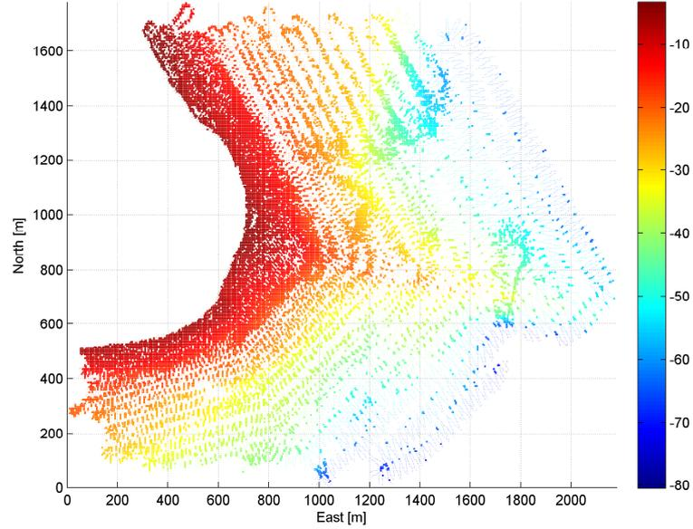
Fig. 6. Data from the survey mission to the Espalamaca converted to a matrix layout. The origin is located at latitude  $38.5379^\circ$  and longitude  $-28.6097^\circ$  with a resolution of  $1254 \times 1536$  for an area of  $H = 1779.6m$  height by  $W = 2180.8m$  width.
