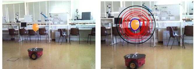
Fig. 2. Real time target tracking. Left: Experimental setup; Right: Target identification, where the initial snake is presented in black, its temporal evolution is presented in red, and the contour final estimate is presented in blue.
