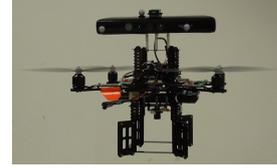
Figure 8. The *AscTec Pelican* equipped with a *Microsoft Kinect*, a *Microstrain 3DM-GX3-25* and the *VICON* markers.
