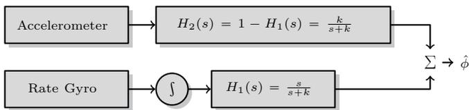
Figure 5: Pitch estimated based on data from IMU using complementary filters.
