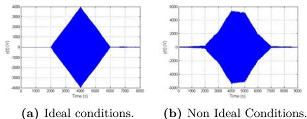
Figure 4: Response of a matched filter to a sinusoidal signal under ideal and non-ideal scenarios.
