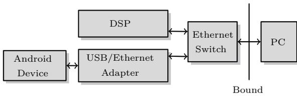
**Figure 11:** Outbound Connection, DSP and Android’s device connected through an Ethernet switch.
