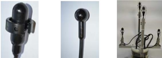
(a) Hydrophone (b) Transducer. (c) USBL array.
