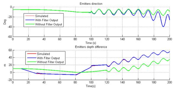
Figure 7: Results of the transmitter's distance and depth difference to the diver when using  $\hat{\theta}$ .
