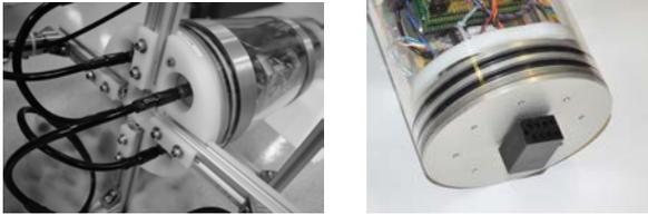
(a) Hydrophones connected through the IE55 connector. (b) SubConn<sup>®</sup> female connector.
