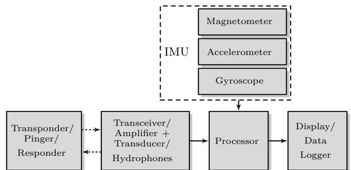
Figure 2: Basic acoustic positioning system architecture.
