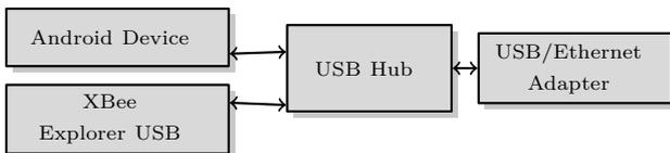
**Figure 12:** Connections established with the Android device.
