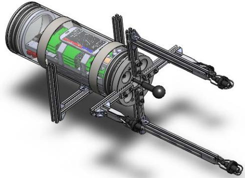
Figure 16: Final prototype of the MAST/AM tool made in SOLIDWORKS<sup>®</sup>.
