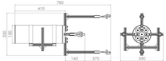
Figure 17: MAST/AM tool dimensions (mm).
