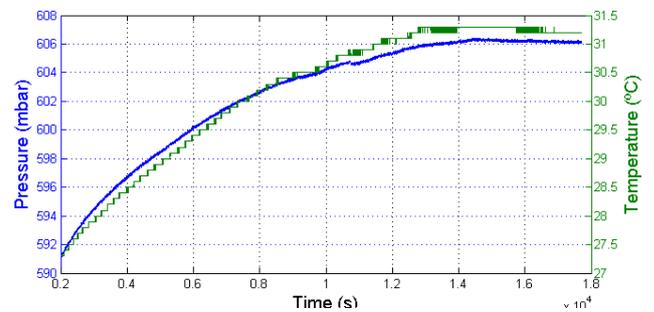
**Figure 13:** Evolution of pressure and temperature values inside the MAST/AM tool.
