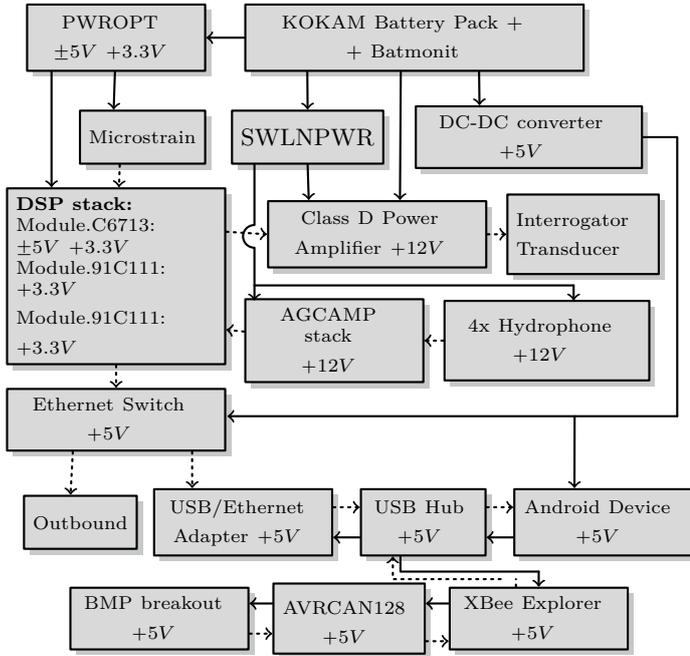
**Figure 15:** Architecture of the prototype for the MAST/AM tool. — power, -- data
