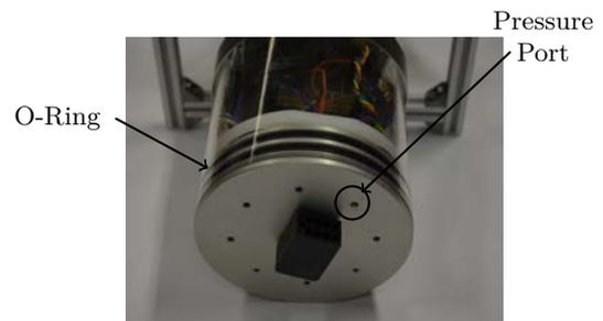
**Figure 14:** O-rings at one end of the MAST/AM tool.
