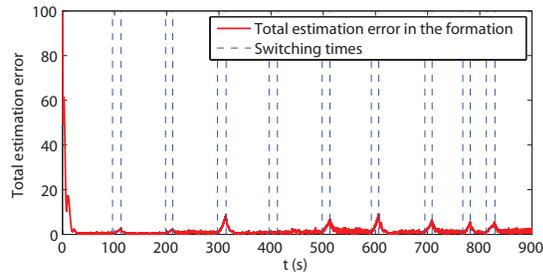
Fig. 2. Total estimation error in the formation, with noise in the measurements
