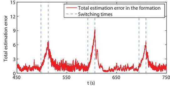
Fig. 3. Detailed view of the total estimation error in the formation, with noise in the measurements
