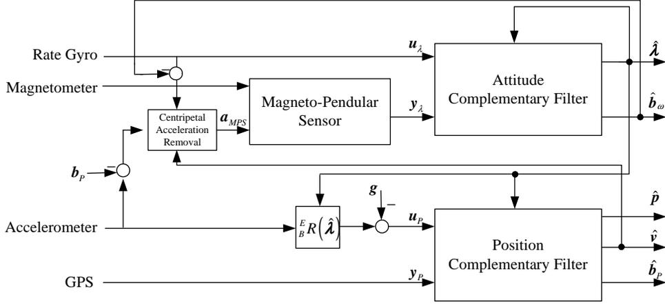
Fig. 3. Navigation System Architecture
