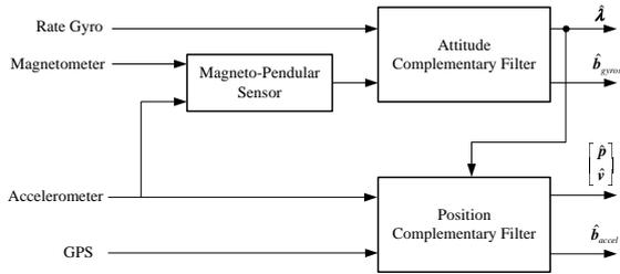
Fig. 1. Complementary Filter Block Diagram
