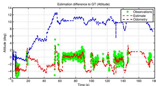
Fig. 11: Attitude Estimate error, relative to ground-truth information.
