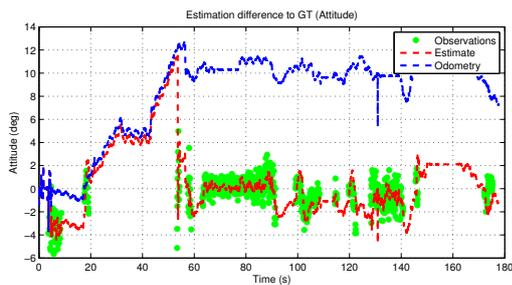
Fig. 7: Attitude estimate error, relative to ground-truth information.
