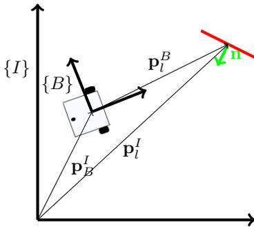
Fig. 2: Schematic of Inertial and Body-Fixed frames
