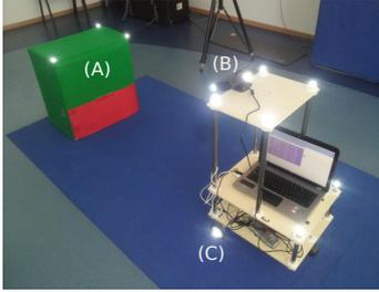
Fig. 3: Biomechanics Laboratory of Lisbon (Landmark (A), Robot prototype (B), Kinect Camera (C)).
