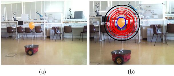
Fig. 2. Real time target tracking. Left: experimental setup; right: target identification, where the initial snake is presented in black, its temporal evolution is presented in red, and the final contour estimate is presented in blue.
