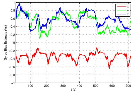
Fig. 7. Detailed evolution of the rate gyros biases estimates
