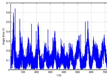
Fig. 8. Evolution of the attitude estimation error using an Euler angle-axis representation
