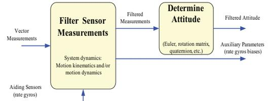
Fig. 2. Sensor-based Attitude Estimation Approach
