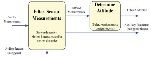
Fig. 2. Sensor-based Attitude Estimation Approach
