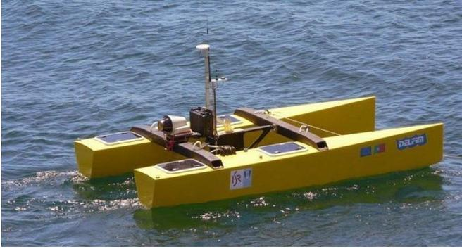
Fig. 1. DELFIMx autonomous surface craft (length: 4.5 m; width: 2.45 m; mass: 300 Kg).
