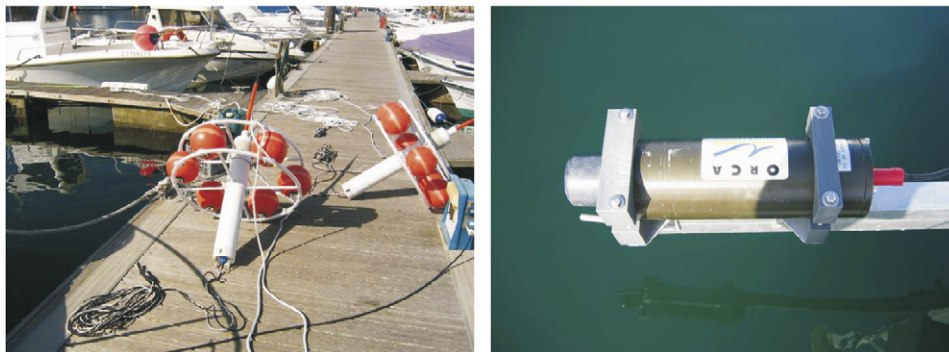
Fig. 10. GIB buoys (left) and GIB pinger (right) (Courtesy of J. Alves).
