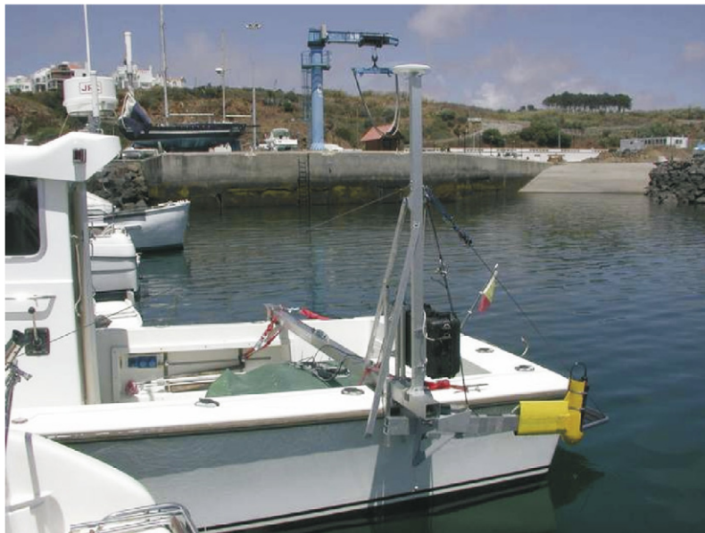
Fig. 9. The IRIS platform with its arm retracted. The yellow unit can be easily replaced with a support for the GIB pinger (Courtesy of L. Sebastião).
