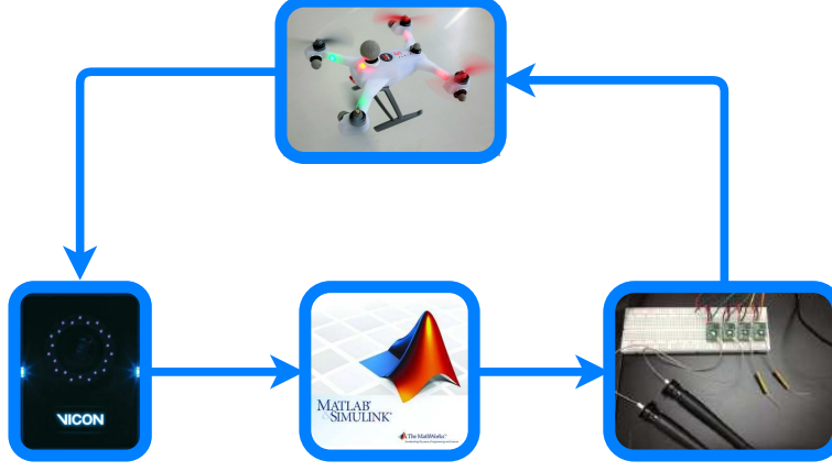
Figure 9. Quadcopter integrated measurement and command architecture.
