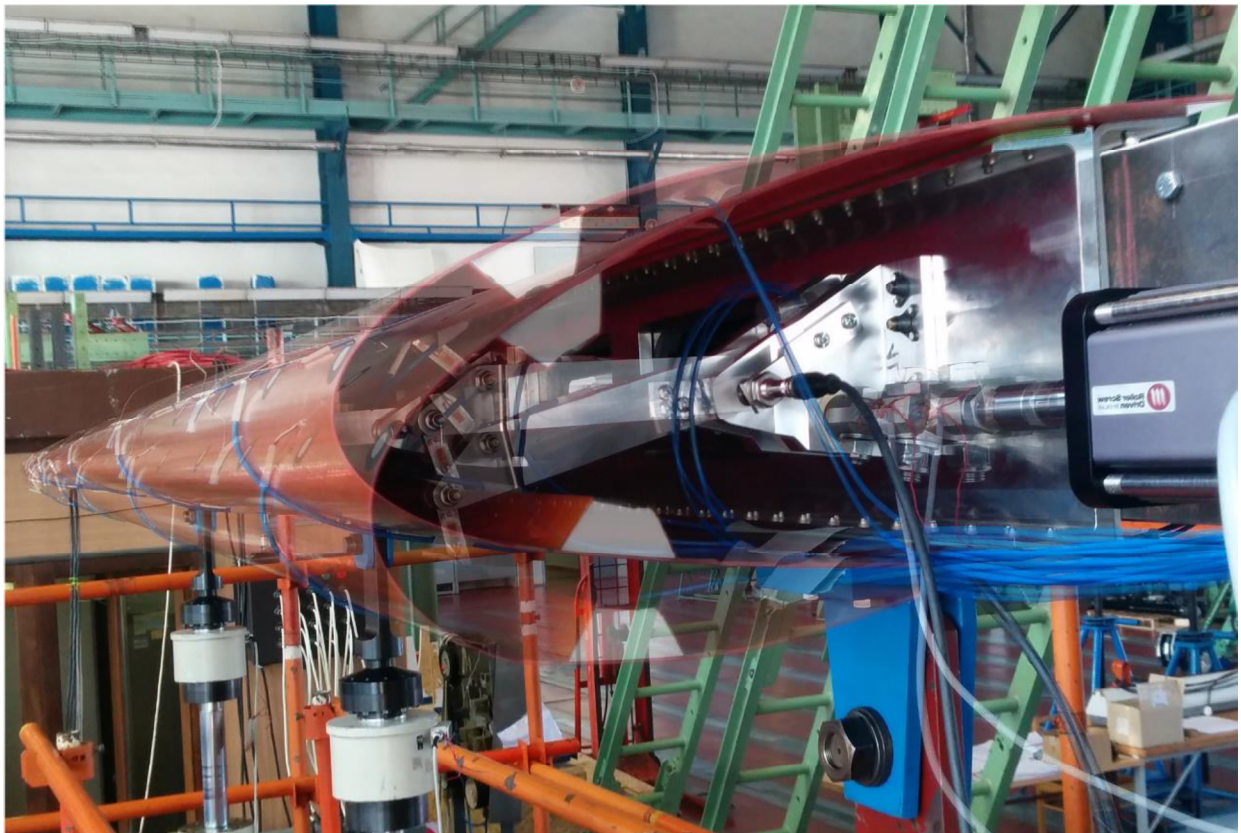
Figure 7: Operation of the developed droop nose at the static test in the facilities of VZLU, Prague
