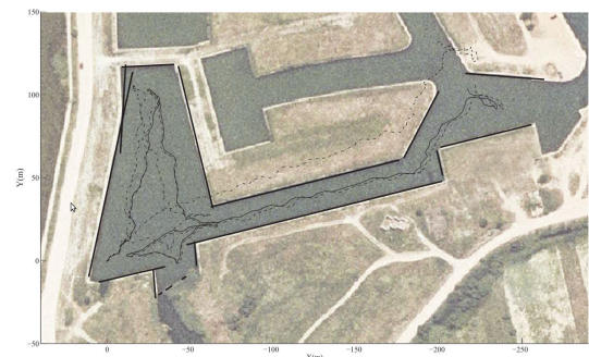
Fig. 2. Example of a line feature based SLAM approach [3]. The image shows the resulting map together with the dead-reckoning (dash-dotted line), GPS (dashed line) and SLAM (solid line) trajectories represented over a satellite image of the scenario.
